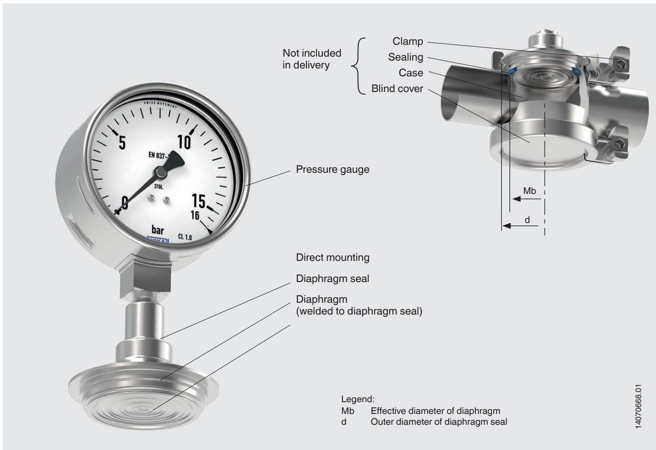
To design the maximum permissible pressure load of a diaphragm seal system at a measuring location, all components <sup>1)</sup> used must be included.
